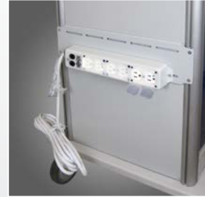
OUTLET POWER STRIP Hospital grade outlet strip. • 15 foot long cord • 6 covered outlets • 15A circuit breaker • UL 1363A rated OS-1
